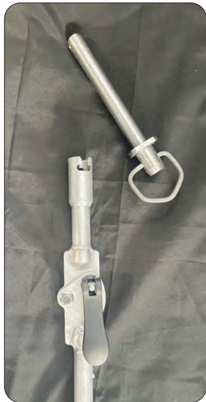
The Drawhand, is a handheld, extendable tool that allows an operator to insert a hitch pin from the cab of a tractor.
