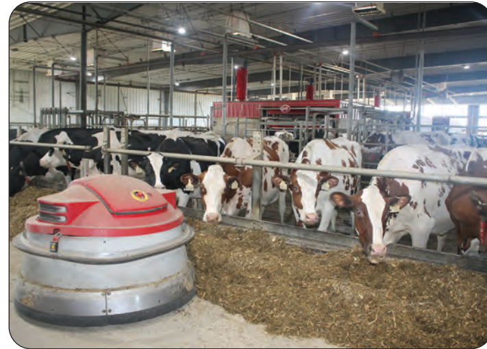
The automated feed pushers ensure food is in close reach for the cows.
