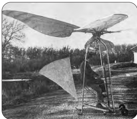
Doug is seen here sitting in his home built aircraft that flies by flapping its wings called an ornithopter.
